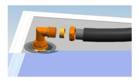
3. For the other collector, assemble 3/4" moufa to the outside thread connector which is on the top of collector. Then assemble the short PEX Black Pipe and Thermal Insulation Pipe. And on the right side of this collector, there are two 3/4" moufa, assemble two union connectors on them.
