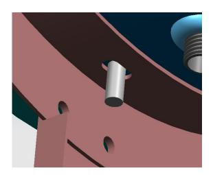
8. Move collector until the outside thread connector on the top of it be toward the 3/4" pipe with 45° on the bottom of Boiler. And connect well the 3/4" pipe of Boiler with PEX Black Pipe.
