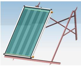
5. Make the left side of the collector mentioned in Step 2, i.e. the side with two connectors, toward the collector mentioned in last step, put it on the support, and push it to the center. When two outside thread connectors touch union connector, fix them. Then set the other Horizontal Strip on the top of Slanting Stands to clip two collectors, but do not fix tightly. Set support plate to the center hole of Horizontal Strip, also clip two collectors and do not fix tightly.
