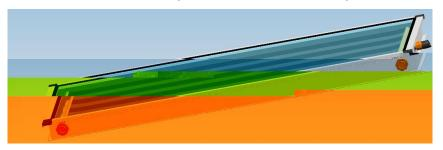
4. Put the collector mentioned in Step 3 on the support as picture, and keep the distance between the right border of the collector and the center of Horizontal Strip to be 15mm.
